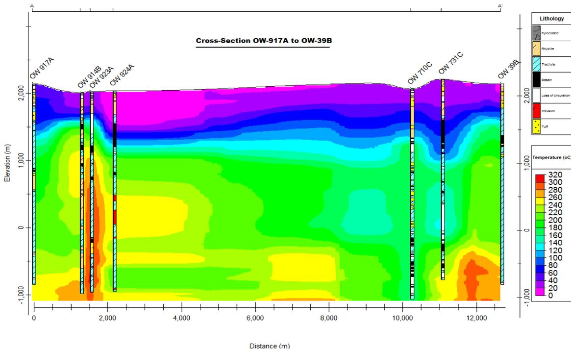
**Figure 4:** A map showing lithology and temperature model cross section A-A'
