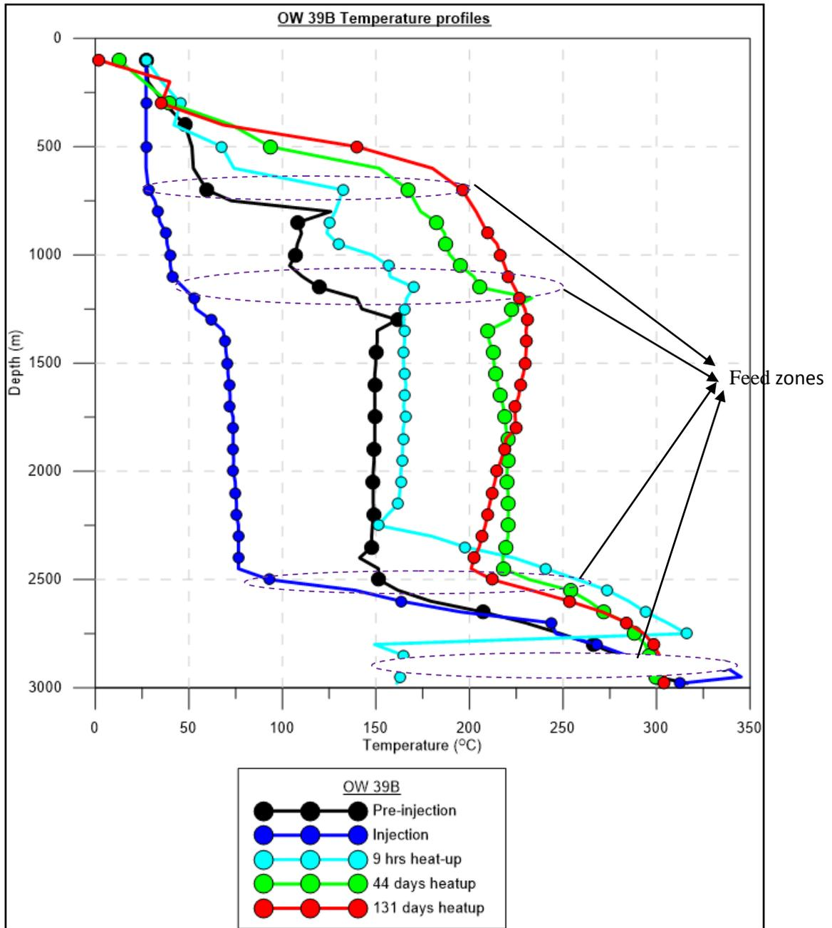
**Figure 11:** Heating profiles and feed zones in purple dotted color for OW 39B
