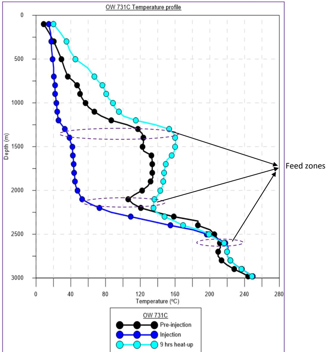
**Figure 9:** Heating profiles and feed zones of OW 731C
