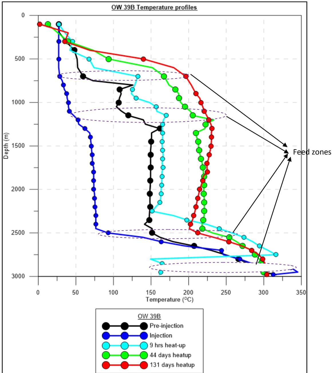
**Figure 14:** Heating profiles for and feed zones in purple dotted color OW 39B
