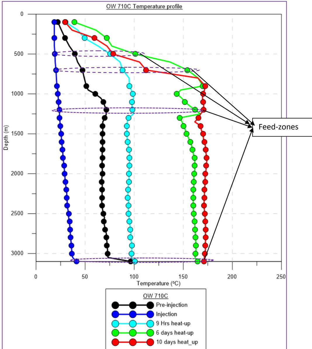
**Figure 13:** Heating profiles and feed zones of OW 710C
