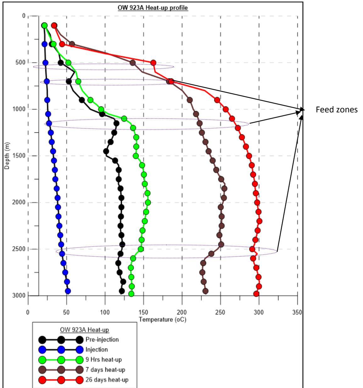
**Figure 6:** Heating profiles for with feed zones marked with blue OW 923A
