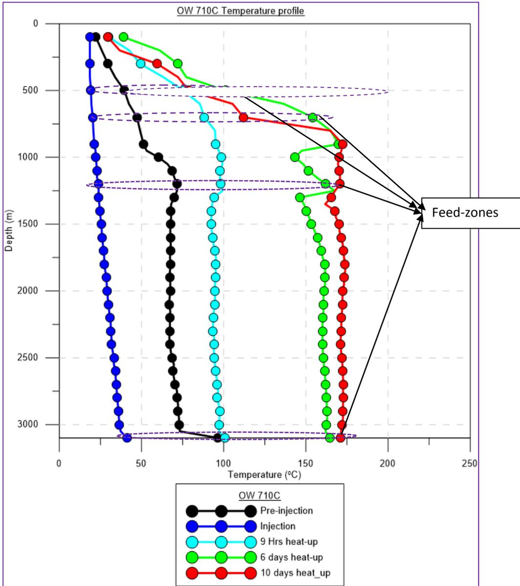
**Figure 10:** Heating profiles and feed zones of OW 710C
