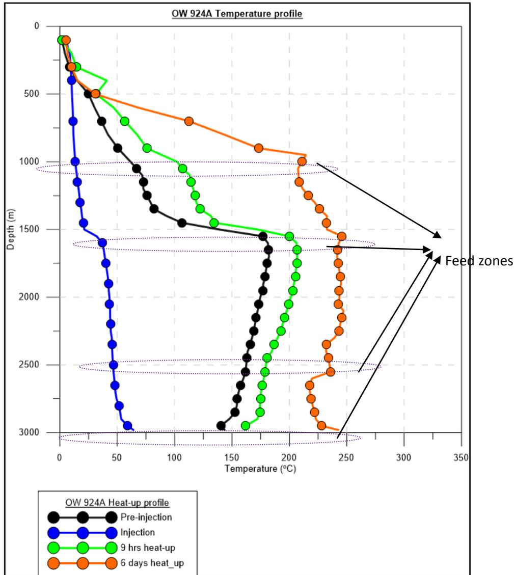
**Figure 5:** Heating profiles for and the location of feed zones of OW 924A
