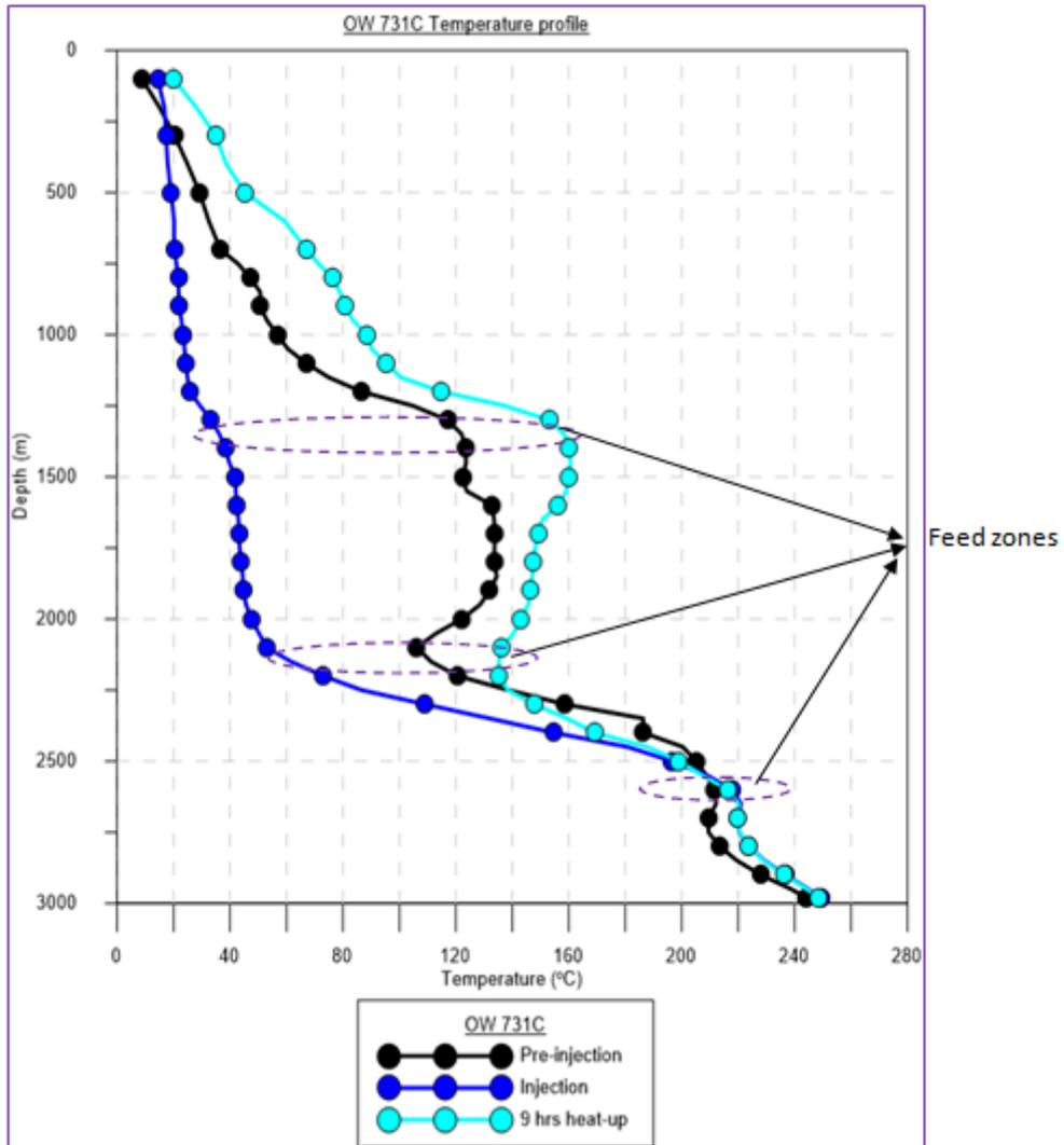
Figure 12: Heating profiles and feed zones of OW 731C
