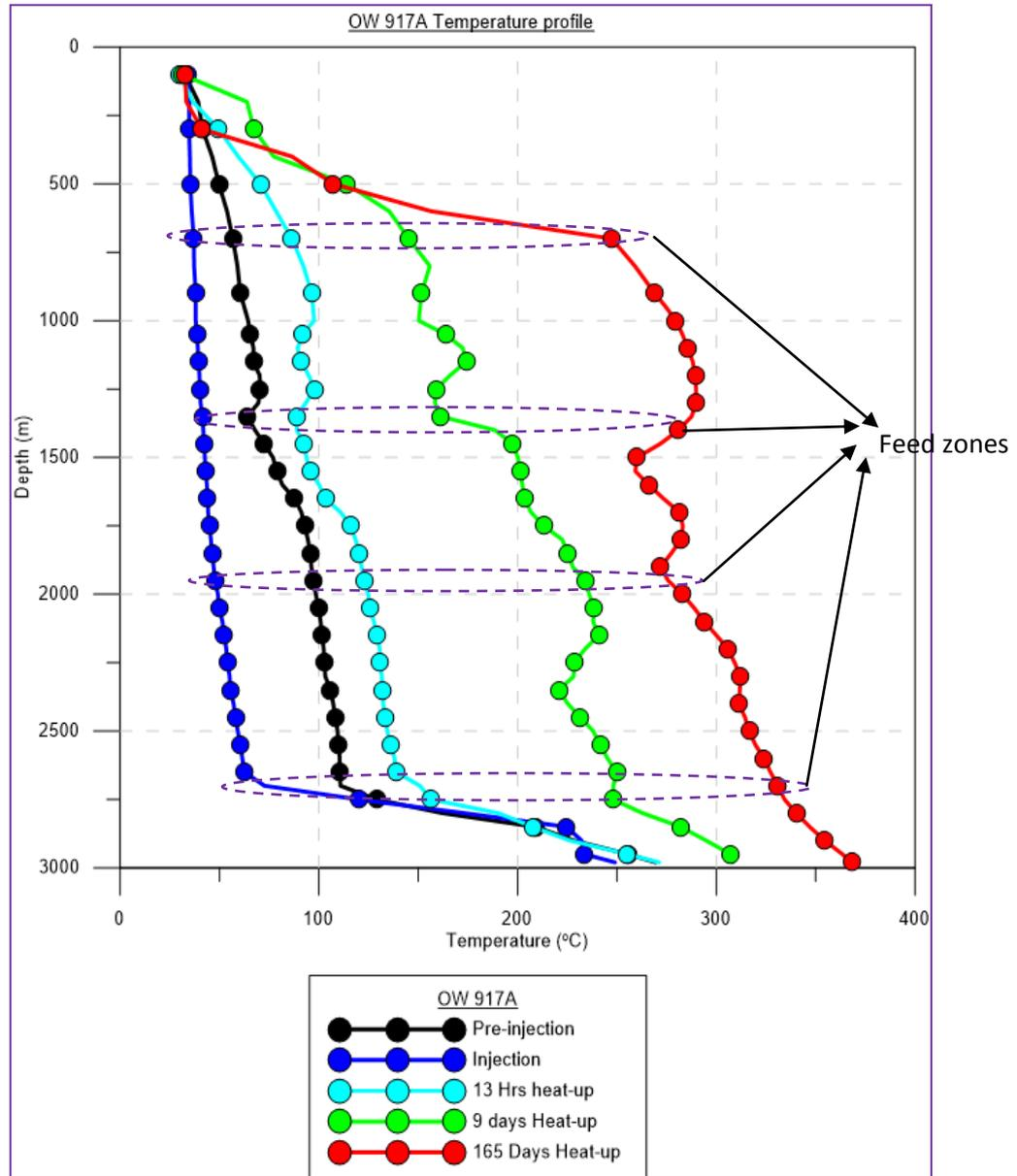
**Figure 7:** Heating profiles and feed zone located with blue color of OW 917A
