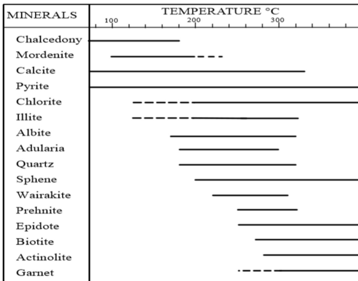
Figure 1: Hydrothermal alteration minerals used as geothermometers and their temperature stability ranges. (Reyes A.G., 1990)
