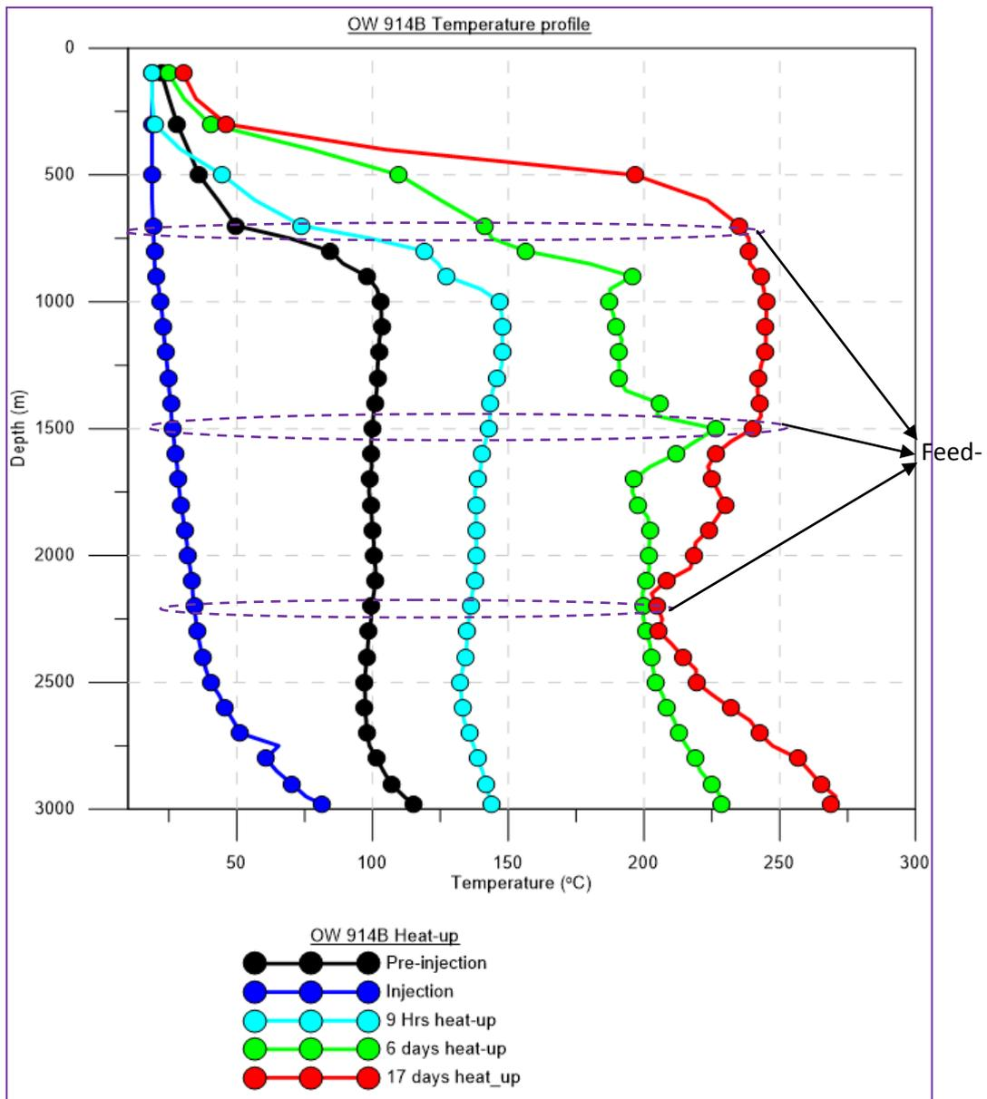
**Figure 8:** Heating profiles and feed zones indicated with purple dotted circle of OW 914B
